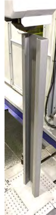
AlSi10Mg 2.0mm \pm 0.2mm Height: 1,160mm Printing time: approx. 11h
