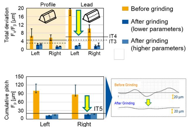
Fig. 2. Investigation of influence of process parameters on the gear quality for internal generating gear grinding.
