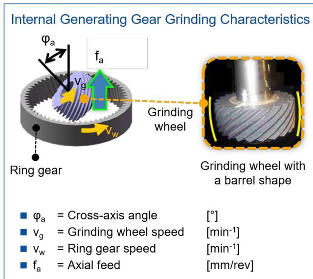
Fig. 1. Operational principle of internal generating gear grinding.
