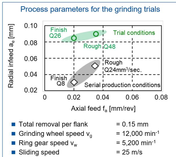
Fig. 5. Description of grinding parameters used in the trials.
