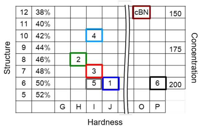
Fig. 4. Grinding wheel specifications for analogy process trials.
