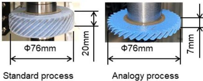
Fig. 3. Grinding wheel dimensions.
