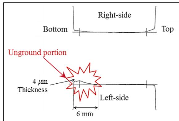
Fig. 10 Gear inspection chart (tooth profile) showing unground material on tooth flank
