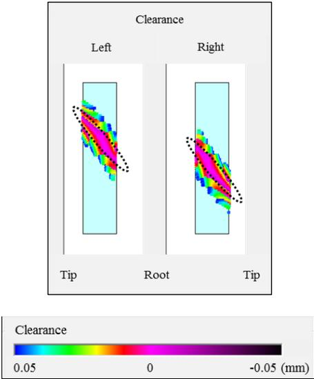
Fig. 6 Region of contact at a given instant (Viewed on flank of threaded grinding wheel)
