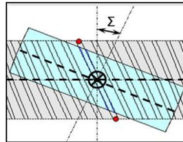
Fig. 4 Initial condition when center of grinding wheel is at the same height as center of workpiece
