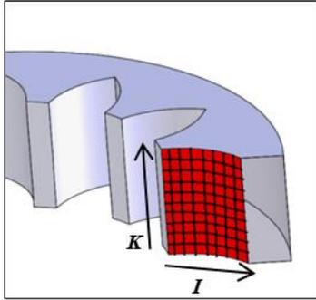
Fig. 2 Grid points on a tooth surface (Left flank)
