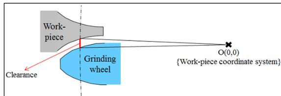
Fig. 3 Clearance between workpiece tooth and flank of threaded grinding wheel
