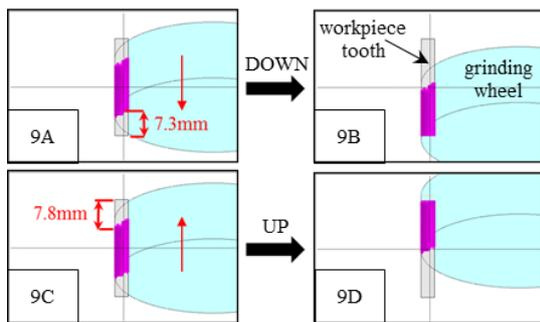
Fig. 9 Estimation of minimum axial stroke using simulation results
