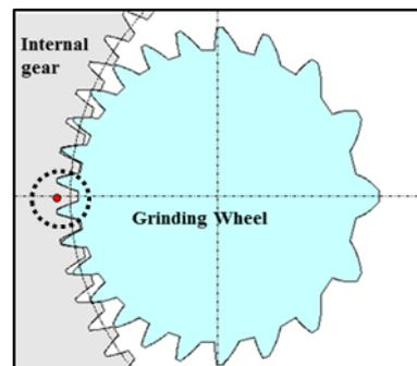
Fig. 5 Initial condition of workpiece tooth and flank of threaded grinding wheel in contact
