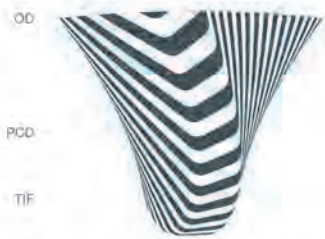
Load concentrated on the edge in the conventional method while in the opposite side thin and long chips are removed so that cutter becomes easily worn.
