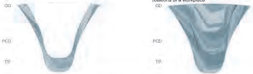
High circumferential feed means chips are removed thickly, so cutting teeth are distributed evenly, reducing wear.
